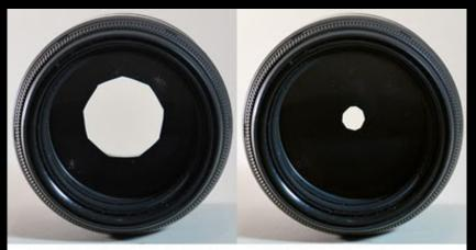
Smaller tistop numbers increase the size of the camera's iris (aperture) opening and decrease the "depth of field" (picture on the left). Larger tistop numbers decrease the size of the iris (aperture) opening resulting in increased depth of field (picture on right).
