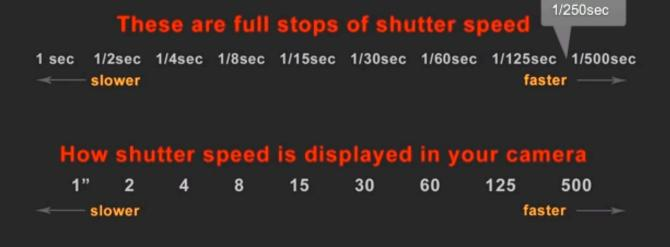
Again, because it is a fraction, the higher the shutter speed number on your camera Actually indicates the faster the shutter is open. For example 500 = 1/500th of a sec.
